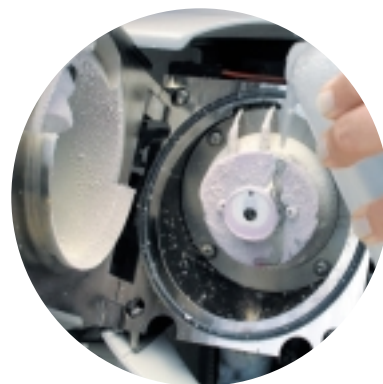
Swing-out spray chamber makes maintenance easier.
